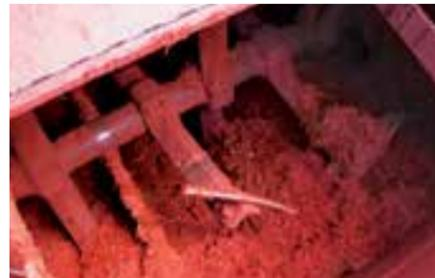
*Ruggedly reliable for extreme-duty operation and easy maintenance, the Sahara employs a solid steel mixing shaft and a bolt-and-key arm and blade configuration.*
